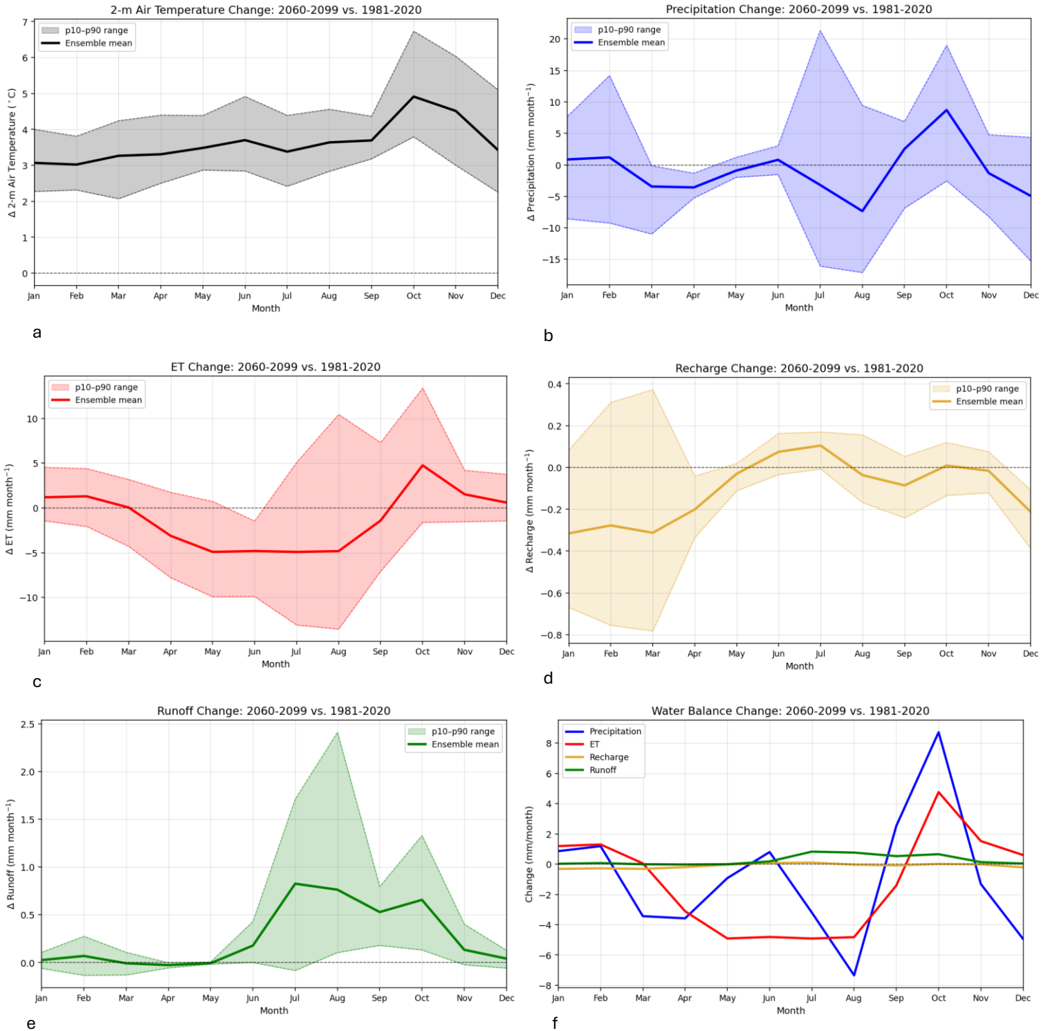
Figure 5. Plots (a)-(e) show projected changes in (a) temperature, (b) precipitation, (c) evapotranspiration (ET), (d) natural recharge, and (e) runoff statewide, comparing end of the 21 st century to the historical record from 1981-2020 under the IPCC Scenario SSP3-7.0. 10 Plot (f) shows the change in the water balance components (P, ET, recharge, and runoff) on a single graph for direct comparison. The analysis uses 14 dynamically downscaled global climate models (GCM) at 9-km resolution and the Noah-MP land surface model. The ensemble mean of the 14 GCMs is shown in bold for each component of the hydrologic cycle, with the 10-90 th percentile shaded to show model projection uncertainty.
